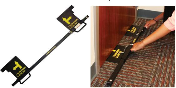
The Barracuda Model DSI is designed to lock down <u>inward</u> swinging vertical doors in a matter of seconds. Simply place the device on the floor and slide the metal plates under the door. Pushing outward on the handles engages the plates to the exterior door jamb and the device is securely locked in place by simply inserting a pin.
