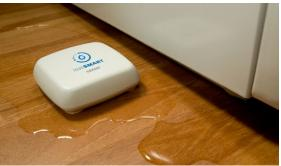
Though a little pricier than some of the other sensors mentioned, the LeakSmart sensor has the potential to save a significant amount of money because it not only detects leaks, it connects to your water main and shuts off all water automatically within five seconds of detecting a leak to prevent the damage from occurring using the LeakSmart Valve.
